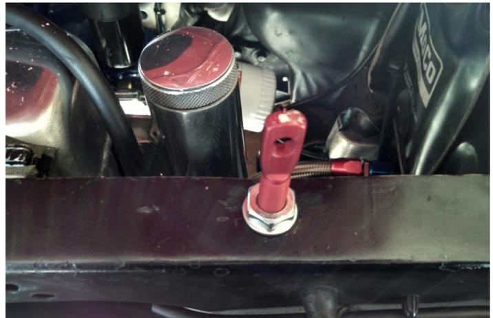
**After the latch posts were positioned, I put a small dab of white grease on the center top of the post and gently brought the hood down to make contact with top of the latch posts. Did I say gently make contact? Yeah, gently!**
