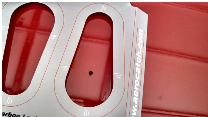
Remove the latch posts for now so you can close your hood and liberally apply a surface of masking tape all around the pilot holes. This tape will allow you to use a good marking pen to trace the mounting templates AND protect your hood's finish from marks from the jig saw or cut-off wheel (I used both). Also, use paper under the hood to catch shavings etc. and keep them out your engine compartment.
